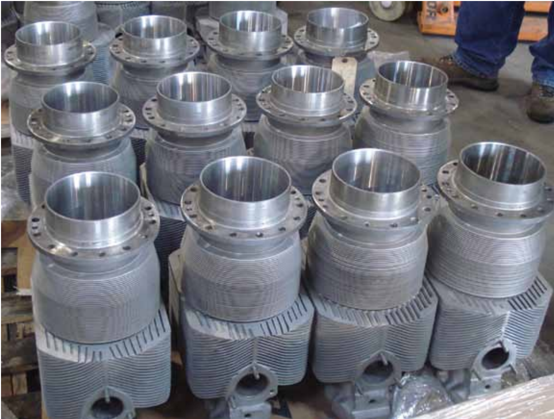
INDIVIDUAL CYLINDERS placed in the staging area for a remanufacturing process at Tecmotiv.
