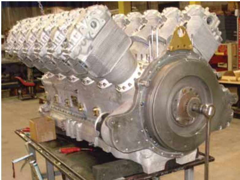
ONE OF THE 12-cylinder engines that Tecmotiv workers disassemble and clean before the remanufacturing process begins.
